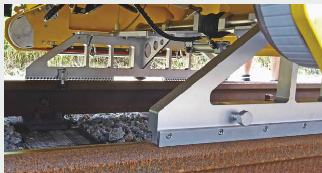
RMF 1100 integrated in reprofiling machine
